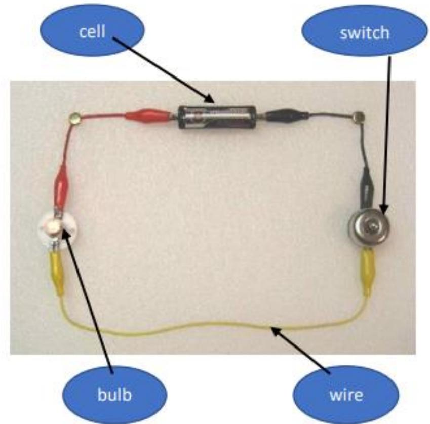
When a **switch** is open (off), there is a gap in the circuit. Electricity cannot travel around the circuit.
