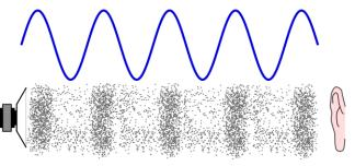
When an object vibrates, it causes movement in the air particles.
